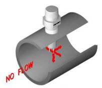
For a no flow condition the thermal differential between the two tips is high because of relatively low heat transfer.
